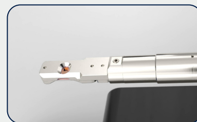
TEM mode (sample on the bottom)
