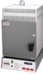
ASPHALT IGNITION FURNACES
