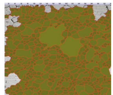
Grain sizing planimetric solution
