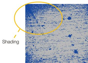
Shading correction produces even illumination across the field of view.
