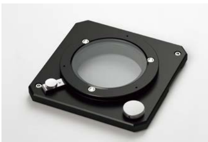
STM7-RS100 for STM7-CS100 100 mm x 100 mm stage
