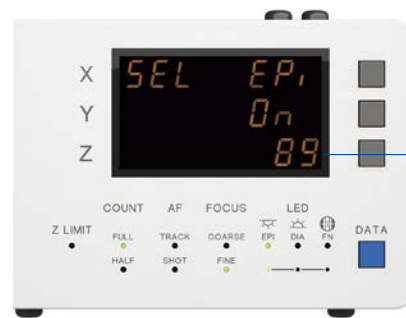
Digital display shows quantitative light intensity
