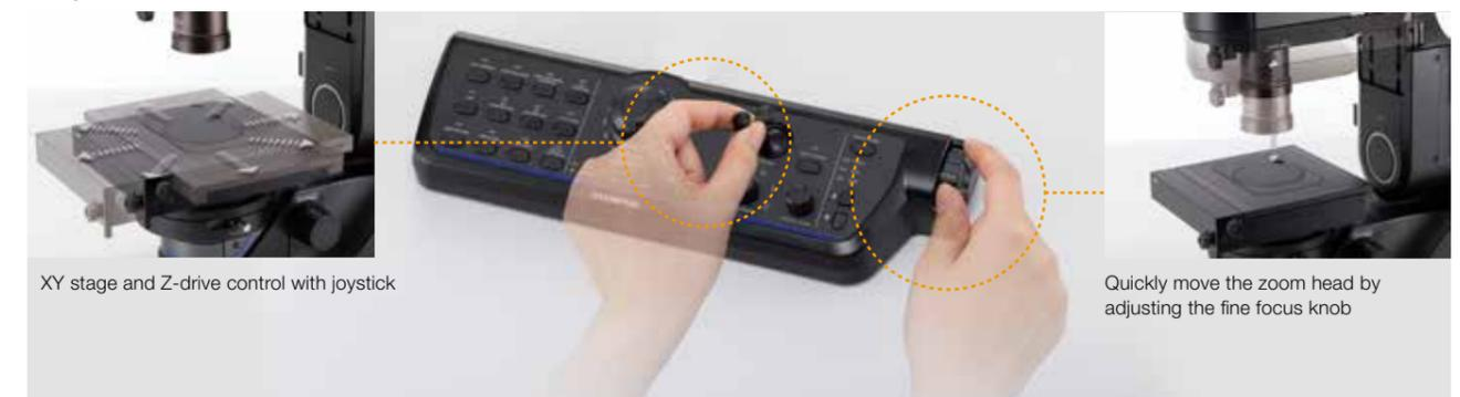
XY stage and Z-drive control with joystick
