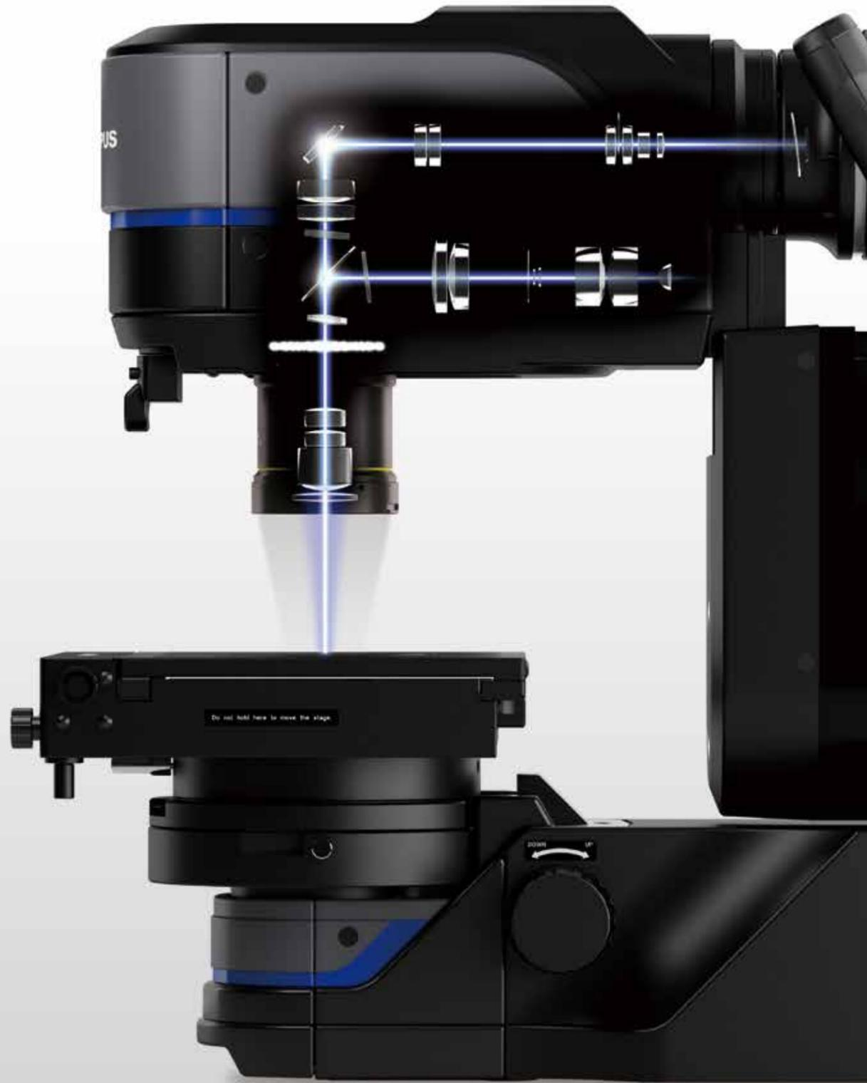
The microscope's telecentric optical system enables you to obtain very precise measurements while the guaranteed accuracy and precision bring confident in your results.
