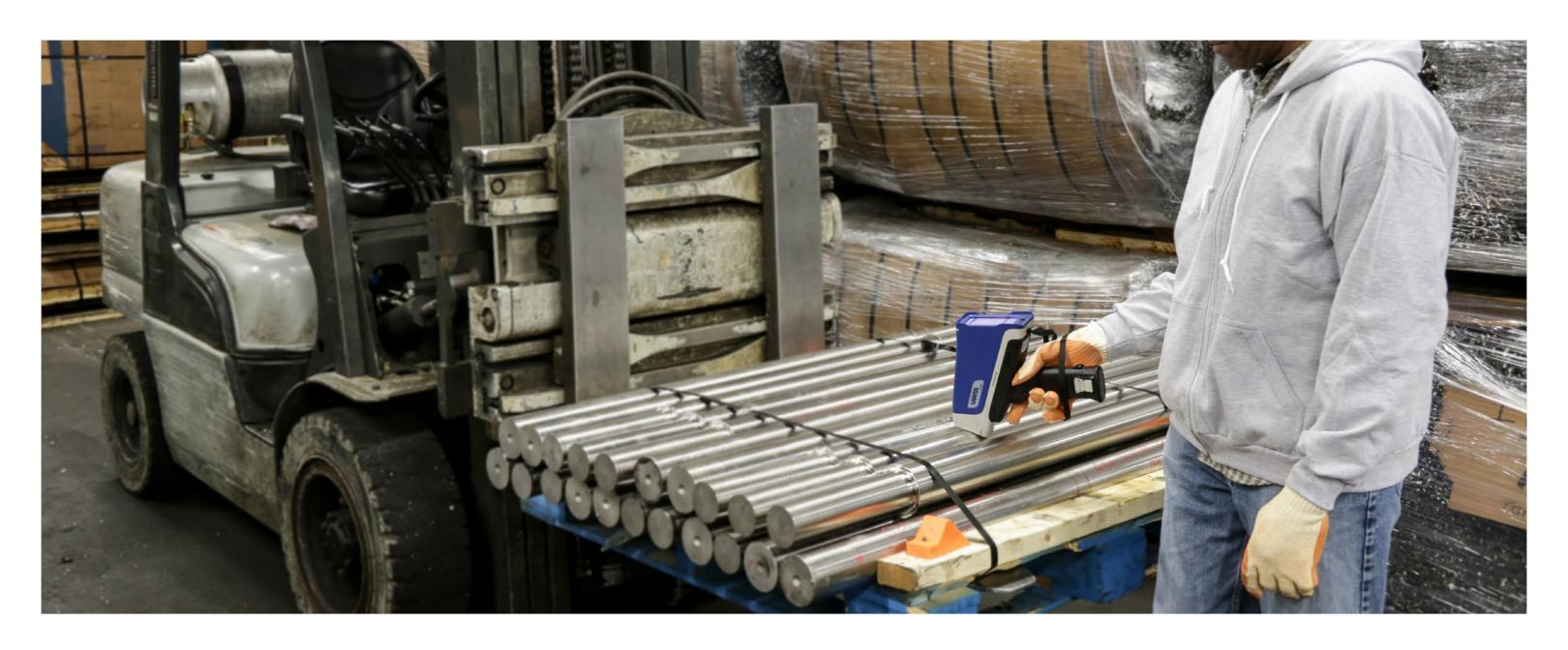
Olympus' Vanta<sup>™</sup> analyzer is our most advanced handheld X-ray fluorescence (XRF) device. These rugged, powerful, and intuitive instruments provide rapid, accurate element analysis and alloy identifications to customers who demand laboratory-quality results in the field.
