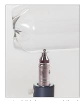
In applications such as plastic containers, simply drop the small target ball inside the container. The magnetic probe held on the outside of the container attracts the target ball. When scanning the probe along the surface or critical corners, the small steel target ball will follow. In the Minimum Mode feature, the gage continually displays both the
