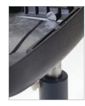
The standard probe along with one of the two target disks and a replaceable chisel wear cap makes the Magna-Mike 8600 gage ideally suited for most automotive tear seam applications where measurements need to be made in a thin channel or groove.
