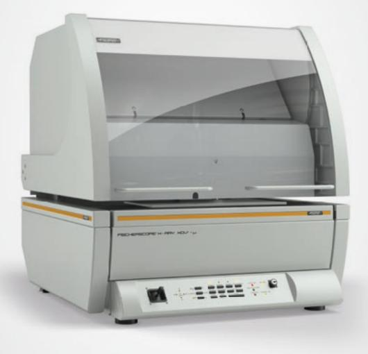
The lead frames used in the manufacture of semiconductor memories have many multilayer coatings – gold, palladium, nickel and copper, etc. Their composition and thickness can be precisely determined using X-ray fluorescence. The specially developed desktop instrument FISCHERSCOPE® X-RAY XDV®-µ LEAD FRAME is equipped with polycapillary X-ray optics for exact measurements on very small structures. This makes it possible to take automatic measurements for quality control purposes.
