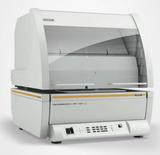
Conventional X-ray instruments require longer measuring times if the structures are very small (< 0.1 mm). Fischer has therefore developed a special measuring device that permits short measuring times even with small measuring spots – the FISCHERSCOPE® X-RAY XDV®-µ. This is due to its polycapillary optics, which is a bundle of hollow glass fibers that strongly focus the primary X-ray radiation. The signal intensity achieved this way enables repeatable results with short measurement times.
