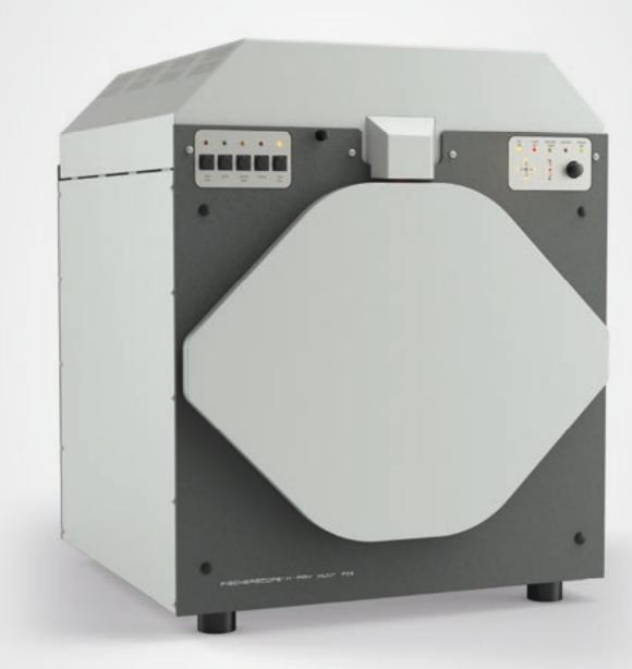
Air absorbs the X-ray fluorescence radiation from elements with low atomic numbers. This is why they are difficult to detect in normal atmosphere. With its FISCHERSCOPE® X-RAY XUV 773, Fischer offers a device with measuring chamber that can be evacuated, to provide a vacuum to measure light elements. For measuring liquids or loose powder samples, Fischer offers a helium option.
