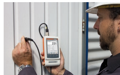
Measurement of paint coating thickness
