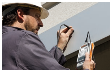
Measurements of anodised aluminum on a façade
