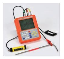
The test is carried out automatically by the BGCMap, which applies a current and records the voltage. The GPS co-ordinates and the date and time of the test are also recorded.polarisation resistance (Rp).
