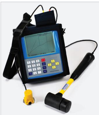
By assuming a wave speed velocity it is possible to calculate the pile length. Reflections can also be obtained from acoustic anomalies within the pile shaft. At low frequencies the response is generally linear allowing measurement of the dynamic pile head stiffness.
