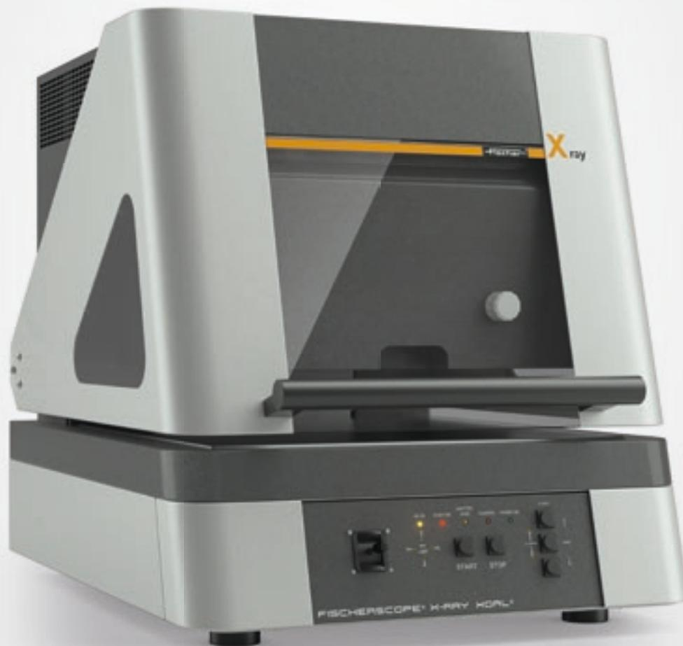
The thinner the layers to be inspected, the more important the choice of detector. The FISCHERSCOPE® X-RAY XDAL® series comprises of several different models. The PIN detector can be used for both material analysis and coating thickness measurement. If ultra-precise analysis is required, the silicon drift detector is the best choice. It offers optimal energy resolution with shorter measurement times.
