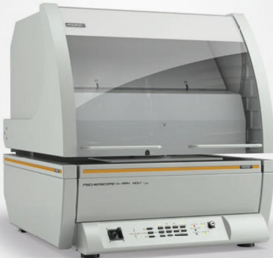
The lead frames used in the manufacture of semiconductor memories have many multilayer coatings – gold, palladium, nickel and copper, etc. Their composition and thickness can be precisely determined using X-ray fluorescence. The specially developed desktop instrument FISCHERSCOPE® X-RAY XDV®-μ LEAD FRAME is equipped with polycapillary X-ray optics for exact measurements on very small structures. This makes it possible to take automatic measurements for quality control purposes.
