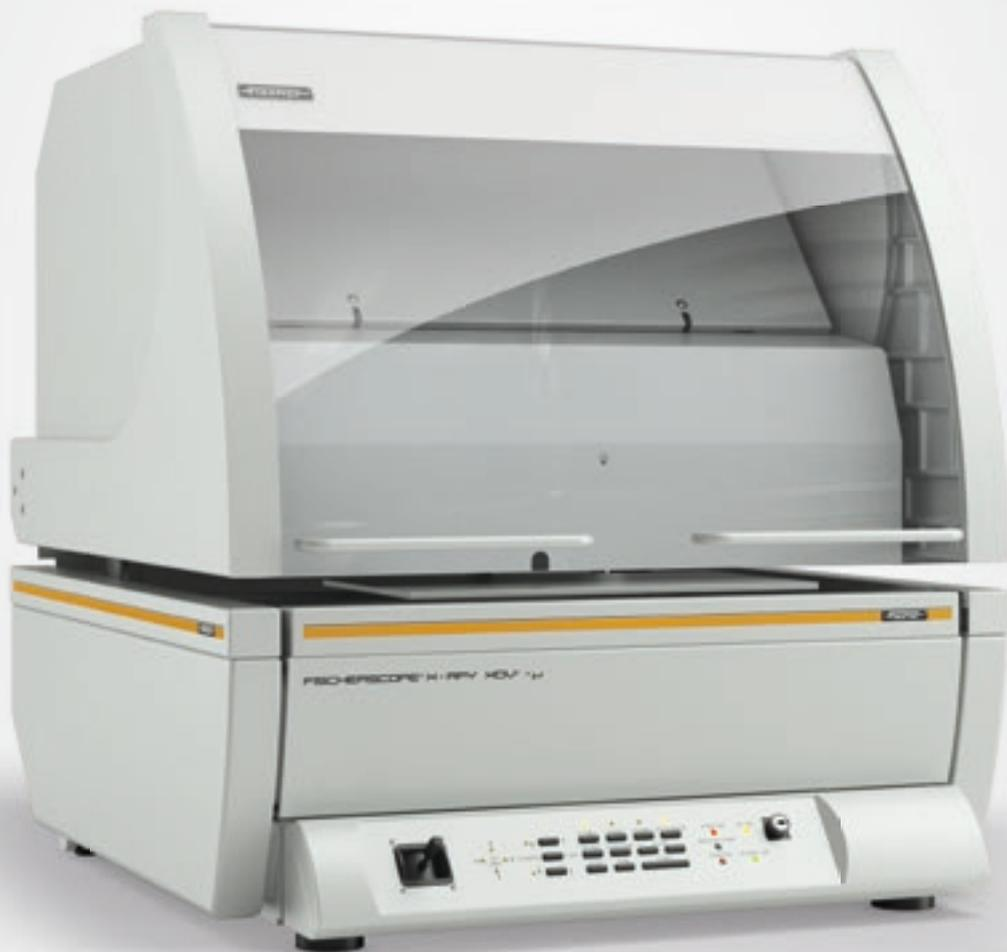
Conventional X-ray instruments require longer measuring times if the structures are very small (<0.1 mm). Fischer has therefore developed a special measuring device that permits short measuring times even with small measuring spots – the FISCHERSCOPE® X-RAY XDV®-μ. This is due to its polycapillary optics, which is a bundle of hollow glass fibers that strongly focus the primary X-ray radiation. The signal intensity achieved this way enables repeatable results with short measurement times.
