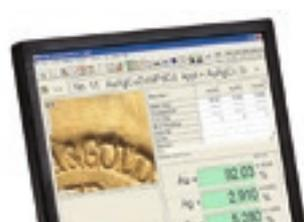
Video image displays the measuring spot exactly
