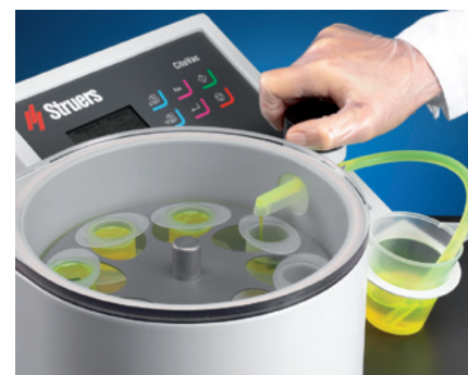
Easy filling of mounting cups
