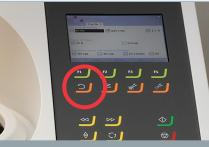
**Remove excess water fast** Press a button, and the disc spins up to max speed to remove excess water from the preparation surface after cleaning.
