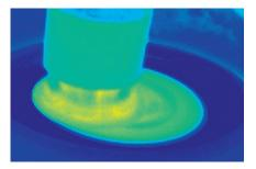
stays low – even with high volume preparation. A nozzle underneath the MD-Disc applies water to the backside of the disc, reducing the temperature by up to 20°. This improves preparation quality and minimizes consumption of suspensions and/or lubricants on the Tegramin-30 and -25.
