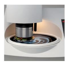
to the bottle and replaces it with water after each OP-step. Struers OP-S NonDry and OP-U NonDry silica suspensions provide excellent polishing results without drying out in the tubes.
