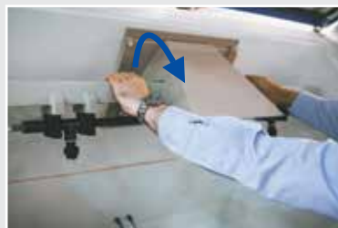
2 The combined air dispersal and oscillating spray bar unit simply lifts out.
