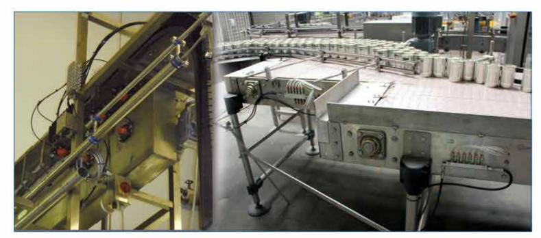
The use of lubrication systems is even more indispensable for the correct operation of machines when they operate in difficult environmental conditions, such as those in the food industry. The installation of an automatic lubrication system allows machine down times to be reduced and allows consumption of the lubricant to be controlled and the life of the bearings, chains and gears to be increased.
