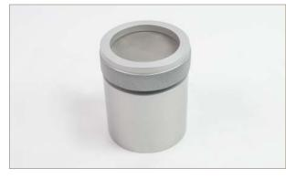
Product Standards: AASHTO T192, EN 451-2, ASTM C430 Stainless Steel mesh, 50 mm internal diameter.
