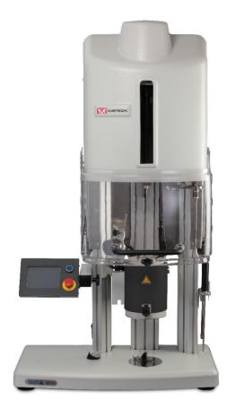
The ability of melted materials to flow under pressure at set temperatures has a fundamental importance in polymer science and technology. The MF50 is especially used by 24/7 laboratories testing several different materials, from fast flowing master batches up to highly viscous rubbery or filled materials, where quick and safe operations have big impact on productivity. It allows multi-weight testing procedures.
