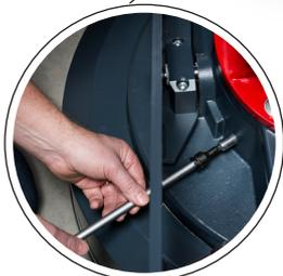
Service 2.0. Loosen three screws to get access to the machine house.
