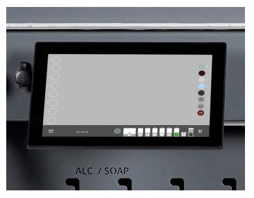
With Xmatic, you get full documentation data in log files that record multiple variables, including the amount of specimen holders that it runs, which methods are used, consumables consumption, and how many hours in service the machine has been running for.
