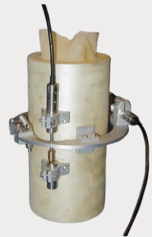
Fig 2. LVDT transducers as shown on sample.
