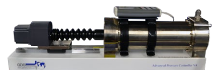
Fig 3. Advanced Pressure Controller used in Unsaturated Testing
