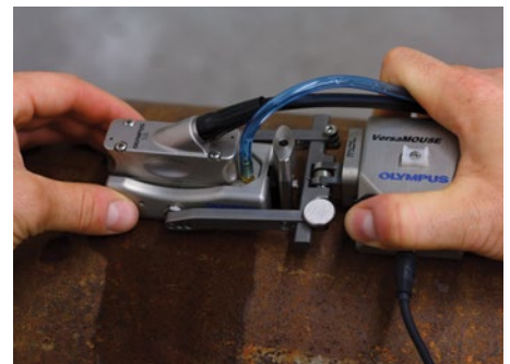
VersaMOUSE and RexoFORM scanners for corrosion inspection.
