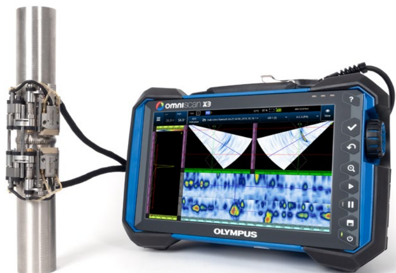
The COBRA scanner on a 0.84 in. pipe with two A15 PA probes with an OmniScan® MX2 16:64 flaw detector displaying two PA groups with sectorial scans and C-scans.
