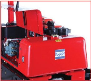
Huge Hydraulic Oil Tank (30 litres) for Longer Interval of Oil Change
