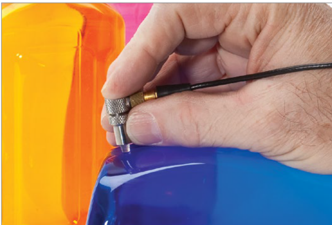
Measure thin plastic material using a 20 MHz delay line transducer.
