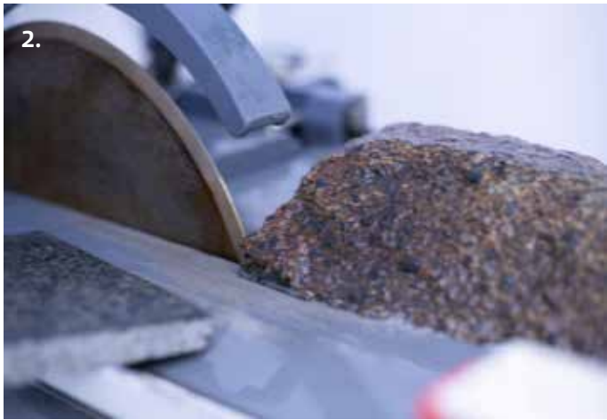
1. GTS1 Thin Section Cut-off and Trim Saw complete with wall mountable control unit 2. Initial stage slabbing & trimming performed on GTS1 saw with slabbing deck 3. Later stage bulk thinning of the specimen
