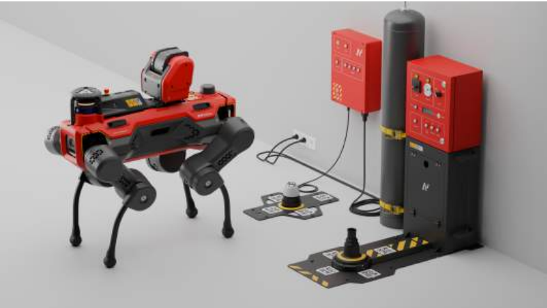
Dock, charger and nitrogen refill station. Floor-mounted installation in a sheltered location in the non-hazardous area. Equipment footprint: approximately 2 × 2 m. Additional site clearances follow the installation requirements.
